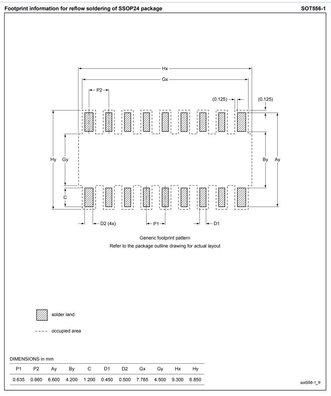
Fig. 2. Reflow soldering footprint for SSOP24 (SOT556-1)
